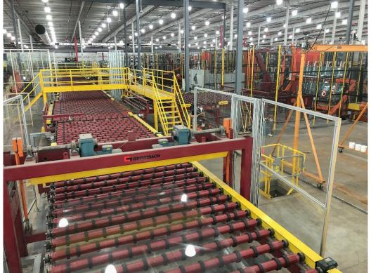
In total, the Mooresville plant consists of one main line, three automatic and seven manual side legs. The three automatic side legs have a total of eight stacking options - the cut flat glass is stacked on racks using direct stackers, swing arm stackers and robots.
